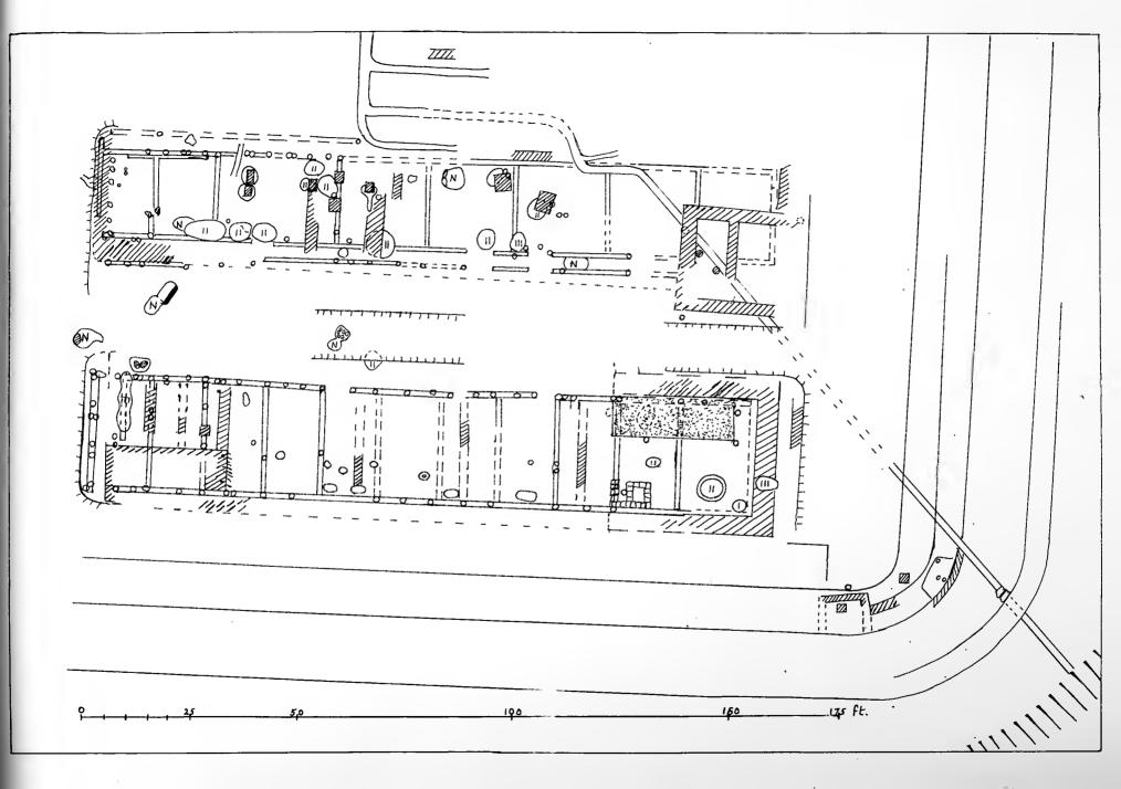
was divided into units 15, 10 and 16 feet (4.58, 3.05 and 4.88 m) wide. From small hearths in the central areas came slag, coal, bar and rod iron, and broken implements. Workshop activity is indicated.
